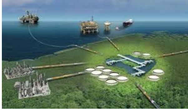
A diagram showing offshore platforms, the actual LOOP station and an offloading ship, the tanks to which the oil is piped, and the refineries that ultimately receive the oil. Loopllc.com.
