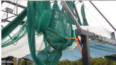
The TED can be seen in the net. Its purpose is to release sea turtles that become entrapped in the trawl. The turtle hits the TED that is tied on
