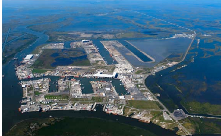
This 2013 photo of Port Fourchon shows Rappelet's Hole full of water and the open water and deteriorated marsh north of the Flotation Canal that has been filled in with dredge materials.
