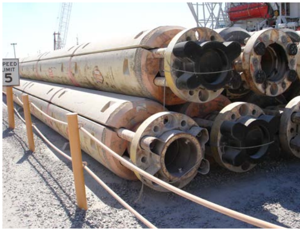
Buoyancy modules that give neutral buoyancy to head drilling risers that extend from the rig to the blowout preventer on the sea bottom.
